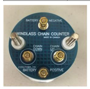
Connections should be ring terminals #6 (3mm) to the brass posts..
